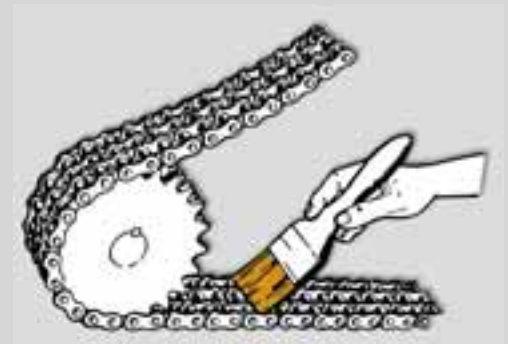
Fig. 3: Chain lubrication by brush
